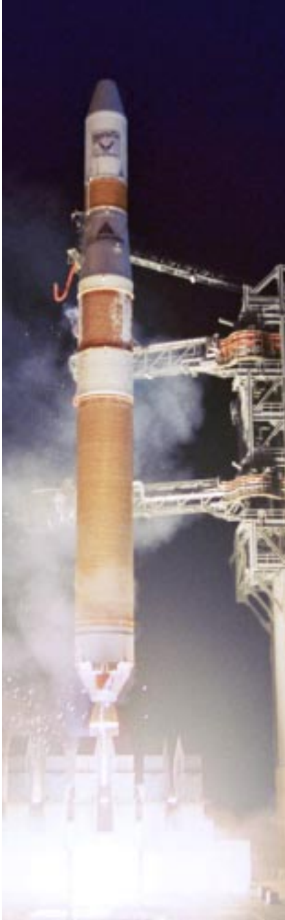
A Boeing Delta IV on March 10 launched the first DOD payload aboard an Evolved Expendable Launch Vehicle. The Delta IV boosted a Defense Satellite Communications System III satellite into orbit from Cape Canaveral AFS, Fla.
